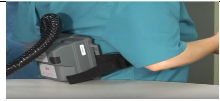
#3 Put on the belt with PAPR box. Fit the box at the small of your back and adjust belt for stability.
