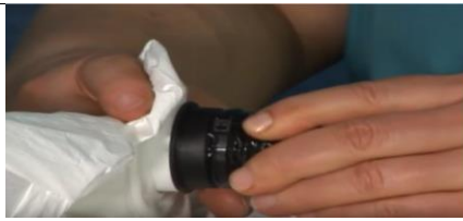
#2 Snap slotted end of the breathing tube into the rear connector of the head cover/hood. Remove protective covering from face shield.
